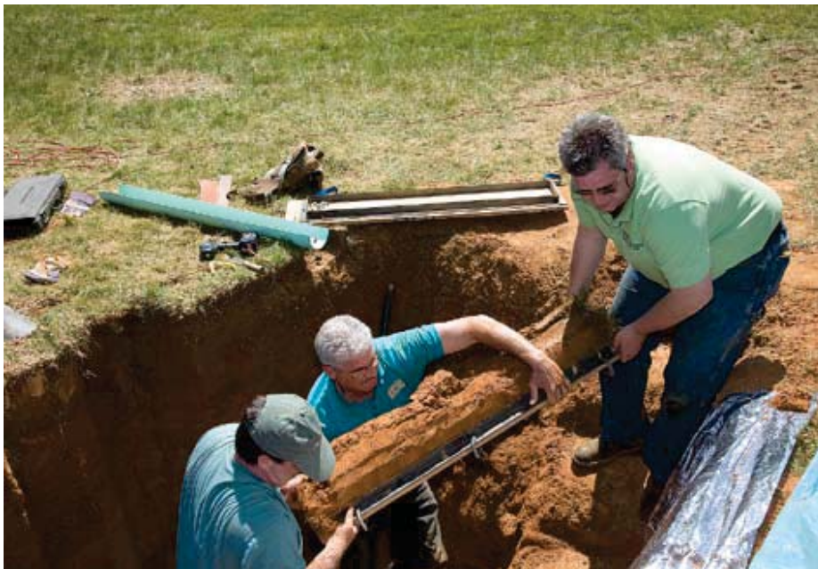
A monolith, or vertical slice from topsoil down to subsoil, preserves a soil’s colors and layered horizons in position. Scientists make monoliths of the important soils in their region and use them in teaching. As they pull the board back, they use strips of cloth to secure the soil to the board. Photo by Donald Hurlbert, Smithsonian Institution.
