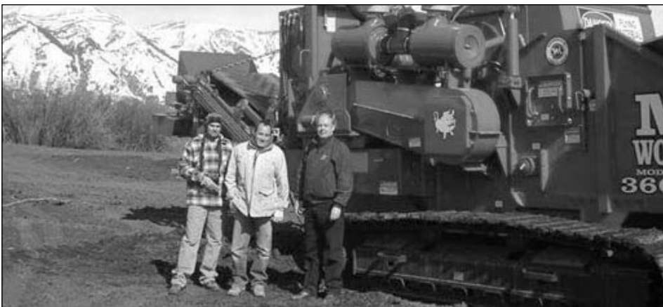
Conversion of biomass to compost in Teton County, Wyoming, is a big job. Dane Buk, owner of the local company Terra Firma, has been awarded the contract for county biomass work overseen by the Teton Conservation District. He recently acquired this Morbark 3600 horizontal grinder on tracks. It is operated by remote control and is capable of whole tree grinding. It can grind 30 to 60 tons per hour, depending on material and the size of screen used. Shown here are (from left) Travis Eva of Trees-R-US, Dane Buk of Terra Firma and Randy Williams, executive director of the Teton Conservation District.
