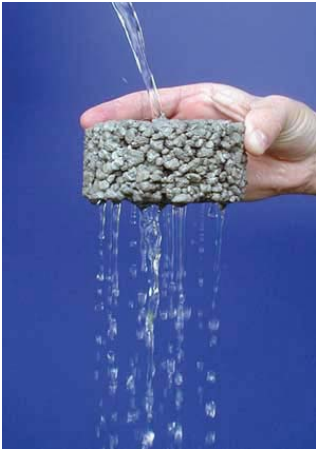
Pervious Concrete in action Photo by: Daily Commerce News & Construction Record
