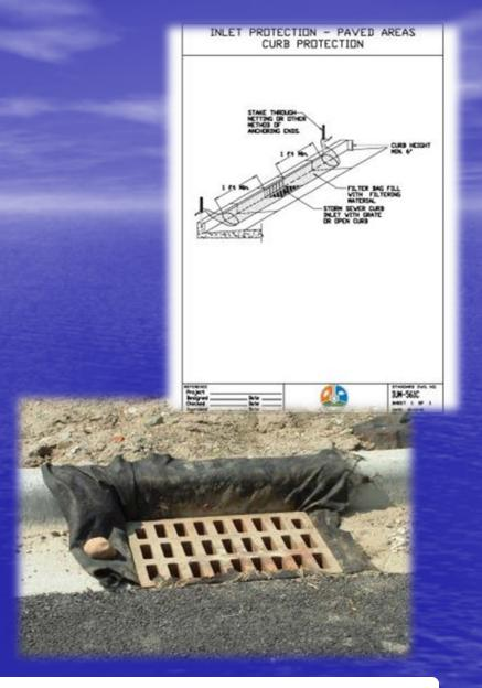
Inlet protection using fabric only as a drop-in shall not be allowed.
