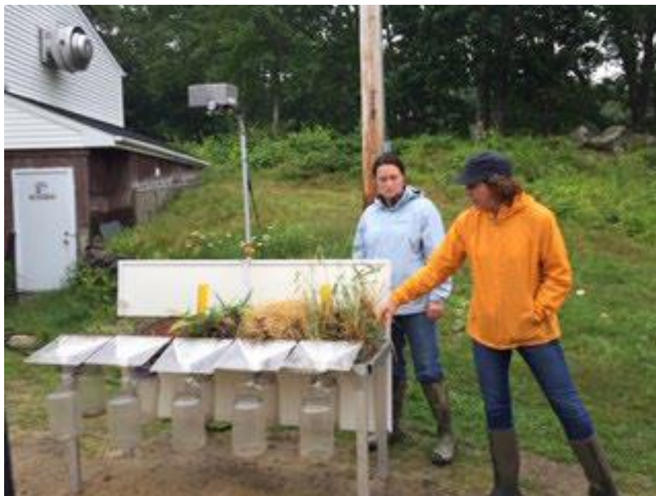
WCCD and NRCS staff explain the various types of cover demonstrated as part of the rainfall simulator (simulator use courtesy of NRCS CT).
